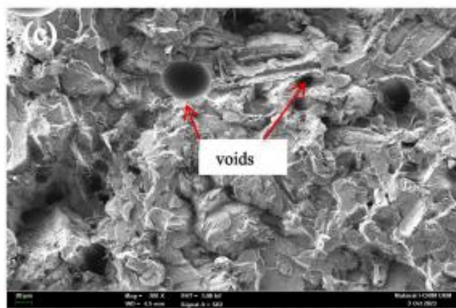
Fig.4.3 (c). SEM micrograph of tensile section failure for bamboo fiber/epoxy composites Voids.
