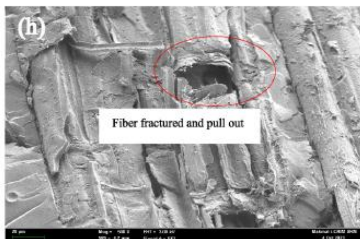
Fig. 4.8 (h). SEM micrograph of tensile section failure for bamboo fiber/epoxy composites Fiber fractured and pull out
