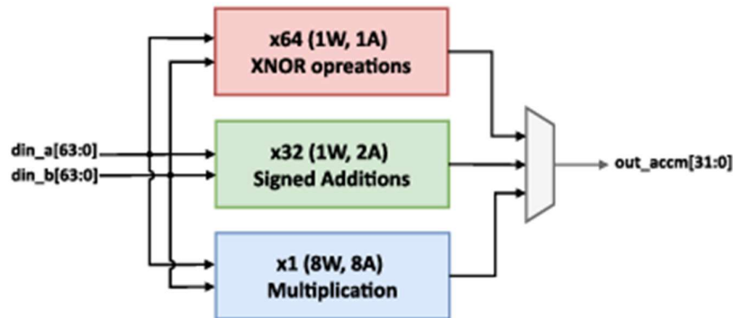
Fig. 10. Baseline-versus-proposed compute concept: precision selection maps the available datapath to binary XNOR, mixed signed-add, or full-precision multiplication.
