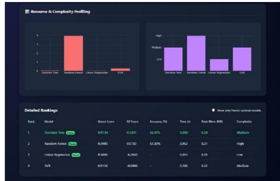
Fig. 3. GreenML Detailed Rankings table for the Uber fare regression task. Models are ranked by Green Score under the Balanced Recommendation Mode. Decision Tree (Rank 1) and Random Forest (Rank 2) are Pareto-optimal with positive R 2 scores. Linear Regression (Rank 3) is Pareto-optimal by energy cost but returns a negative R 2 , making it impractical. SVR (Rank 4) is non-Pareto despite a high Green Score because its R 2 is also negative. The “Show only Pareto optimal models” toggle enables rapid filtering.
